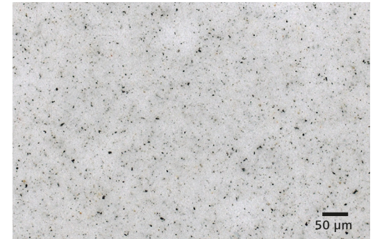
Particle analysis, brightfield, objective: EC Epiplan-NEOFLUAR 20×/0.5
